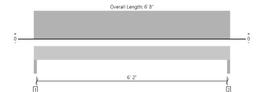
All locations are measured from the outside face of left support (or left cantilever end). All dimensions are horizontal.
