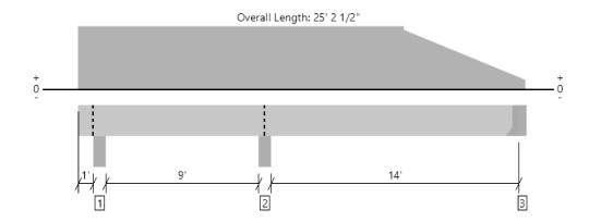
All locations are measured from the outside face of left support (or left cantilever end). All dimensions are horizontal.
